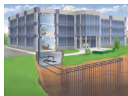
Geothermal closed loop
